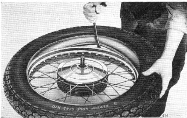
Fig. F17. Levering the first bead onto the rim
