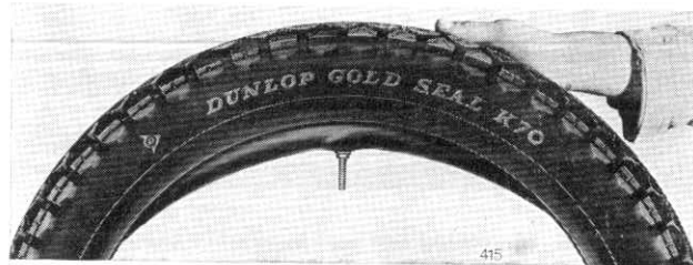
Fig. F15. Cover and tube assembled ready for refitting to the wheel
