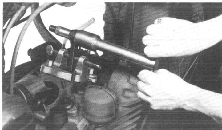
ILLUS. 33 INSTALLING NEW ROD BUSHING
