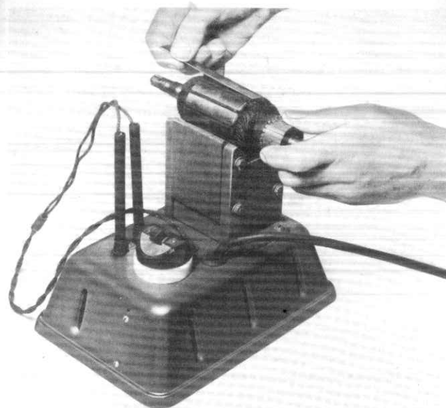
ILLUS. 38 TESTING ARMATURE FOR "SHORT"
