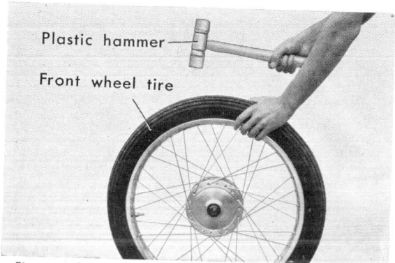
Figure 4-23. Tap the tire all around with a hammer
