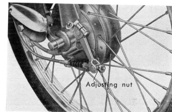
Figure 6-36. Adjusting front brake lever
