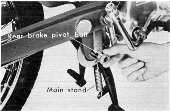
Figure 4-35. Removing brake pedal and stand
