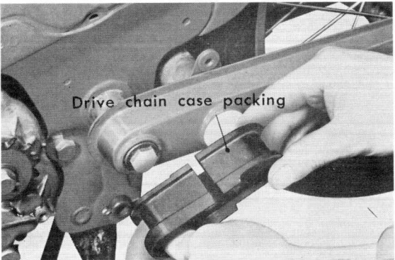
Figure 4-43. Installing chain case packing
