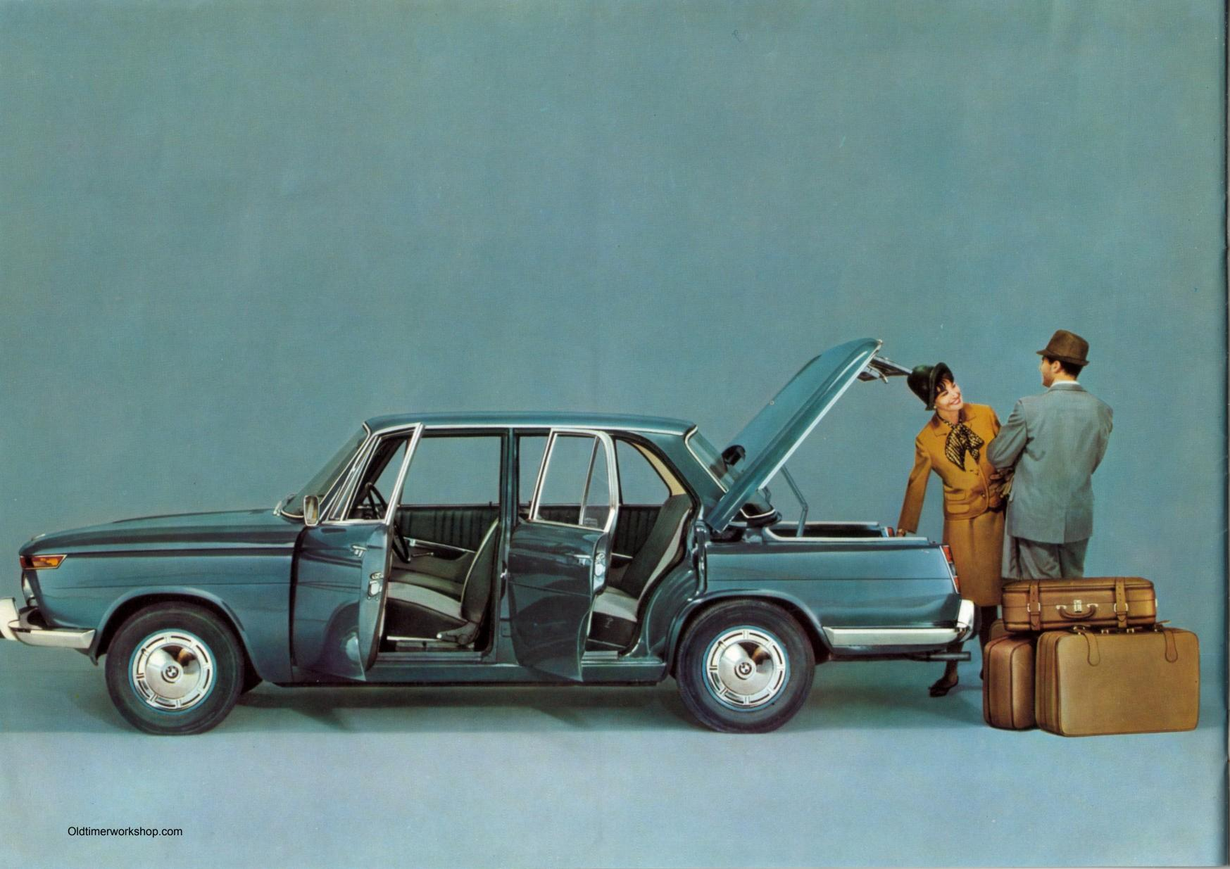
The large luggage boot is neat and tidy, without recesses and corners. Note: The spring-assisted lid. Easy to operate with one hand. The low-level edge makes loading easy. The spare wheel is under the floor of the boot, where it is not in the way, soils nothing, and is yet readily accessible.
